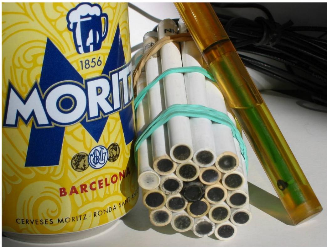
This study analysed several brands of beer by applying a new concept in analysis systems, known as an electronic tongue. / Manel del Valle
